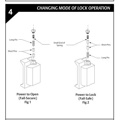
To change electric strike's mode of lock operation, remove brass screw from top of strike body.
