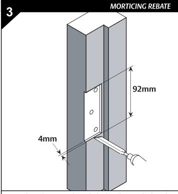
• Using the markout as a guide, neatly chisel out the recess for the strike .
