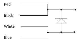
Red and Black joined and to Power Supply. Blue and White joined and to Power Supply.
